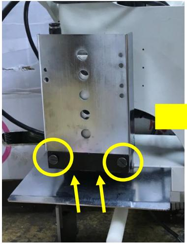
5. 安裝上刀具, 圖上兩顆螺絲可調整刀距 To adjust distance of the cutter by the screws.
